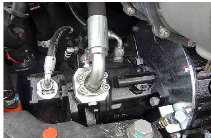
↑ The hydraulics of the machines are usually composed of parts from the major component manufacturers. This gives you more options if something is broken on the machine. The parts can usually be repaired at the nearest hydraulic workshop or, alternatively, the part can be purchased as an original part from the component manufacturer. The picture shows the main pump of the Bobcat, one of the widely used Bosch Rexroth pumps, Type A10VO71. The Bobcat pump is labelled as a Doosan spare part with the identification number 401-00327.
