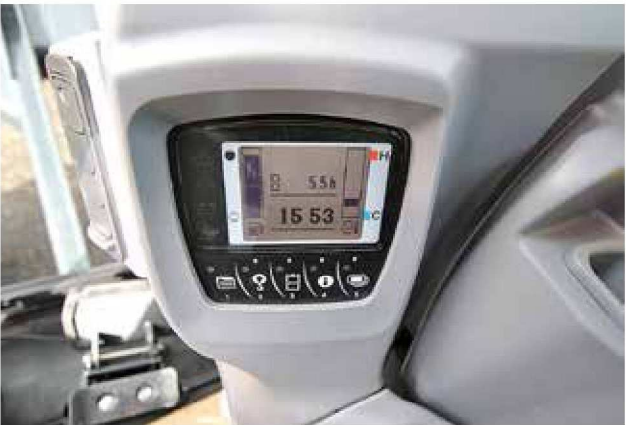
The Kubota display is at the smaller end of the scale. The small, black-and-white and outdated display is reminiscent of excavator displays twenty years ago.
