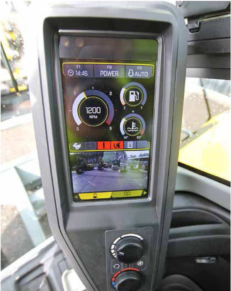
There were big differences in the display sizes. The largest is the colourful and easy-to-read display of the Wacker Neuson. The machine also comes with a reversing camera.
