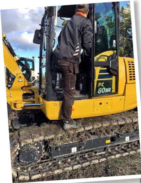
The Komatsu door opening was by far the narrowest. Larger operators have to manoeuvre themselves awkwardly.
